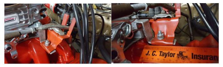
I then cut the original kickdown in the vertical section and welded in a ~5" section in to extend it.
