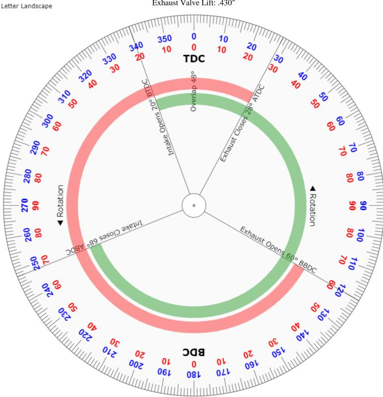
Intake Centerline: 114° ATDC Exhaust Centerline: 106° BTDC
